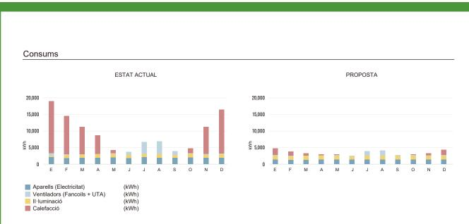
Figure 24. Energy demand of AMB Headquarters before and after the renovation. Image provided by AMB.
