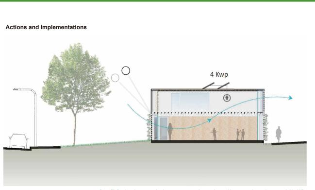
Figure 70. Profile of the center with indication of cross-ventilation and renewable energy production. Image provided by AMB.
