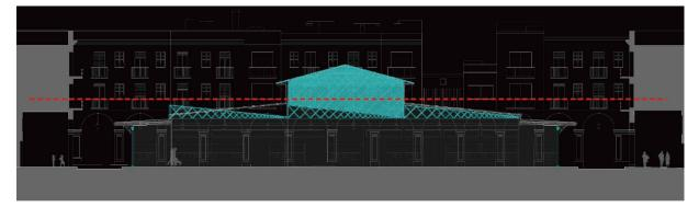
Figure 68. Proposed market building design, with eliminated middle section volume colored in blue. Image Image provided by AMB.
