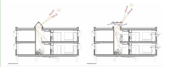
Figure 30. Profile of the Carrer El Pla showing vertical openings for ventilation. Image provided by AMB.
